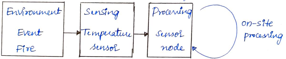
Event detection using an on-site processing
